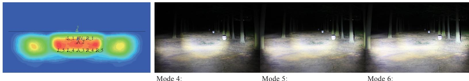
Starting from Mode 4, the wide beam is on. You even have different widebeam selections depending on how much brightness you need. This user-friendly feature can adapt to different riding conditions. The width of the wide beam is three times wider than the German regulation, which provides a wider and clearer vision while turning, and thus increases the security. It provides the user with reliable riding experience.
