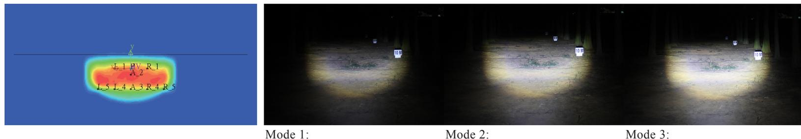
We design the low beam based on German regulation StVZO. With numerous tests and modeling, we successfully obtained the German approval. The key of the regulation is to have a clear cut-off line. Offering great brightness on the road but at the same time, the light should be friendly to opposite people.
