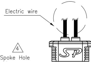
$\triangle 4$  Spoke Hole  $\phi 2.7^{+0.1}_{-0.05}$  - PCD $\phi 50$
